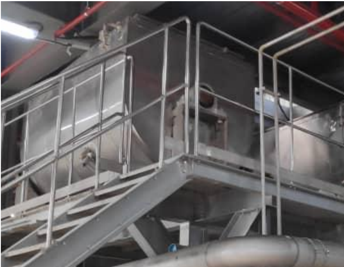
Anti Caking Mixers with Jacketed Cooling Water, Screw Feeders + Chemical Dosing
